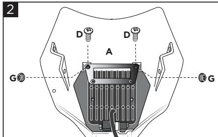
**Tighten the top bracket to the headlight (A) using the screws (D) and the nuts (G).**
