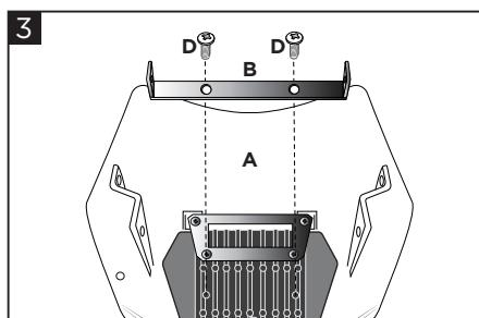
**Tighten the central bracket (B) to the headlight (A) using the screws (D).**
