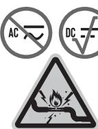
**EN** - The headlight only works in direct current so for **carburetor** motorcycles follow the connection instructions exactly.
