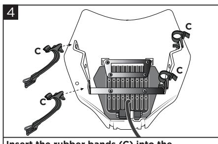
**Insert the rubber bands (C) into the corresponding holes. Check that are mounted as shown in the figure.**
