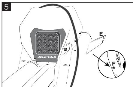
**Place the headlight on the bike and slide the cable, then apply the spoiler (E).**
